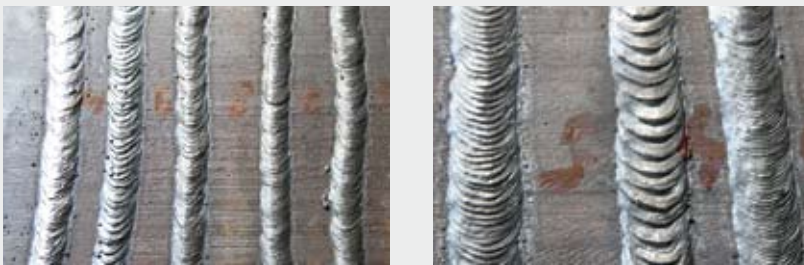
Fig.B Appearance of deposits made with cellulosic electrode
