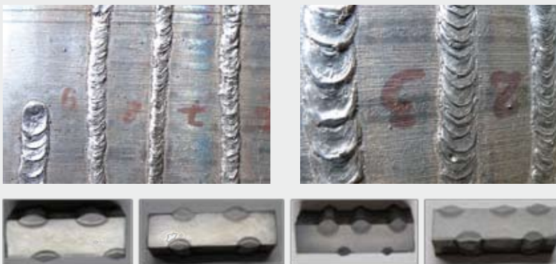
Fig.B Appearance of deposits made with cellulosic electrode
